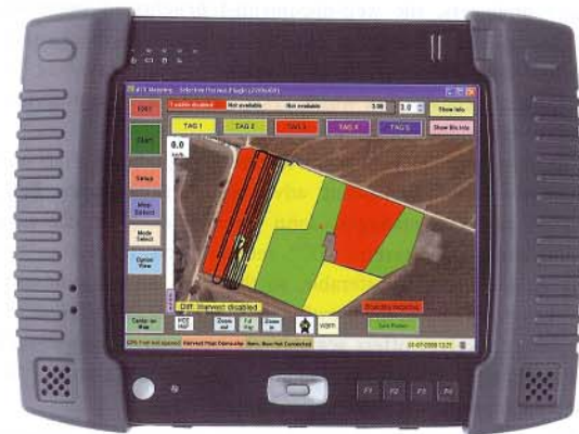
An example of the yield mapping software displayed on the Ultra Mobile Personal Computer, available from Advanced Technology Viticulture.
